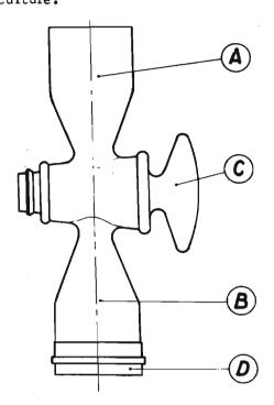
In the diagram, D is a metal filter that does not allow the passing of the eggs. A and B are open-ended identical chambers, and C is a simple stopcock.
